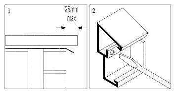
**3.** Starting at eaves, the dry verge sections should be nailed through the fixing slots into the projecting slate. Ensure that the closer overhangs the eaves by the same amount as the first slate course. Slates at the verge should alternate standard slates and slates-and-a-half.
