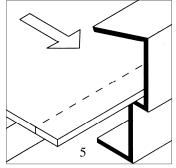
**6.** The ridge cap fixing bracket, with the bolt protruding outwards, should be over inserted into the dry verge and then withdrawn slightly into the opposite side.
